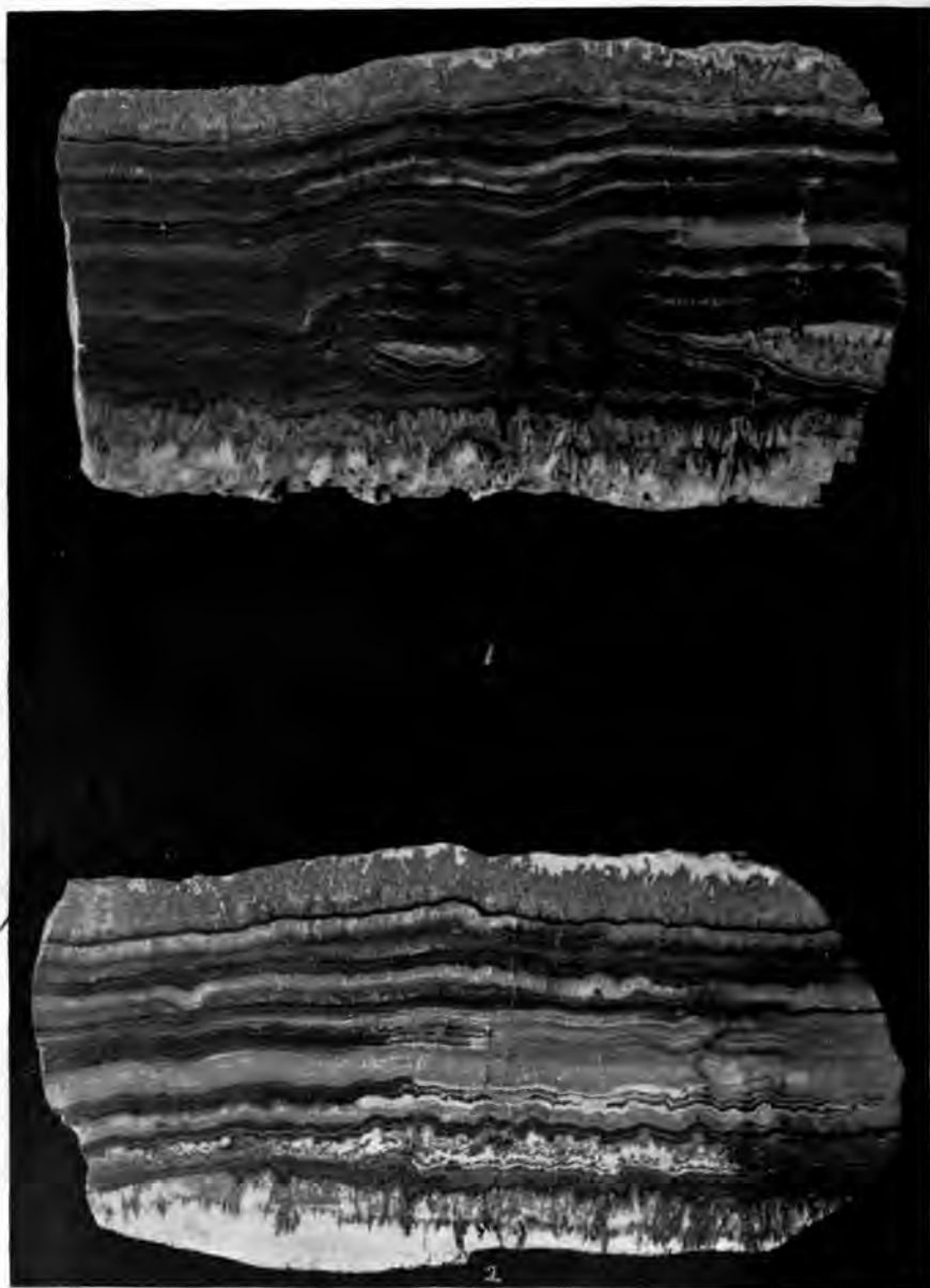
SLABS OF ONYX MARBLE CUT ACROSS PLANE OF DEPOSITION TO SHOW BANDING.
